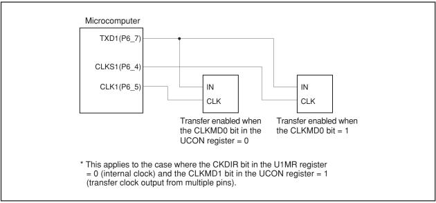
Figure 14.15 Transfer Clock Output From Multiple Pins
